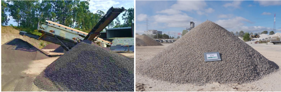
Fig. 8. Steel slag aggregates from electric arc furnace (left) and recycled slag aggregate (right). Reproduced with permission from Ref. [96] under the terms of CC BY 4.0 license. © 2022 C.D.A. Loureiro et al.
