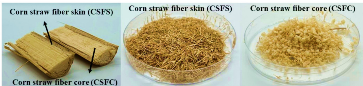
Fig. 7. The appearance of corn straw fiber skin (CSFS) and corn straw fiber core (CSFC). Reproduced from Ref. [93] under the terms of CC BY 4.0 license. © 2022 Z. Qi et al.
